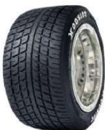
CIRCUIT RADIAL WET
